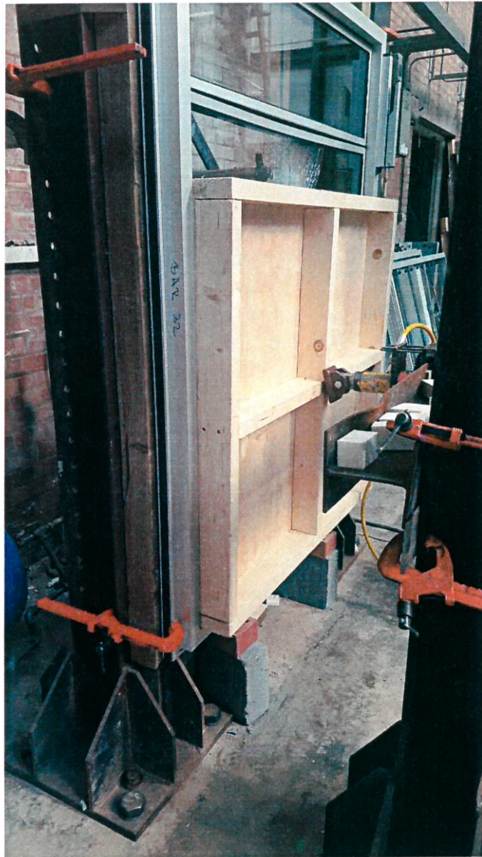
Plate 3 - Generic Test Arrangement Uniformly Distributed Load
