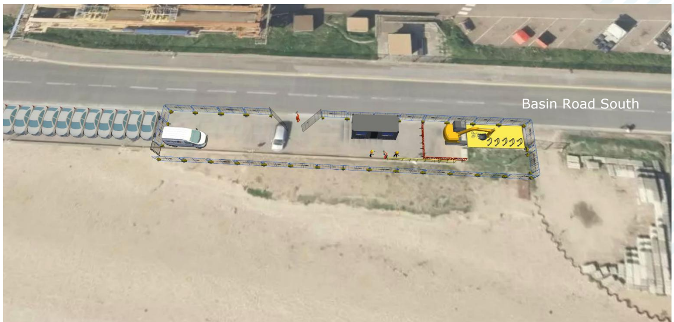
Figure 2 Area 2A Works Layout Sketch showing easternmost enclosure. The fenced enclosure will progress westward as the works proceed.
