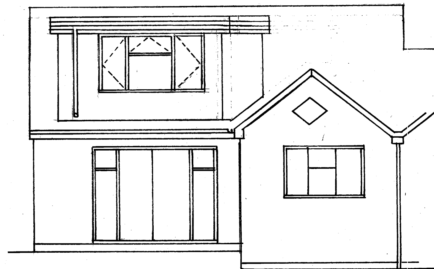
REAR ELEVATION (WEST) 1:50 AT A1
