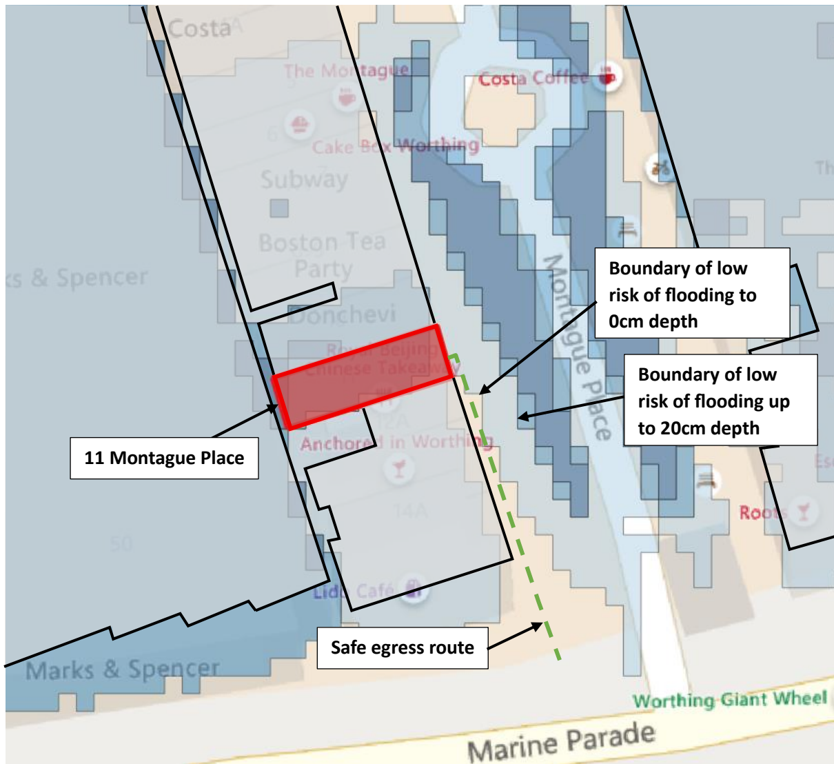
Extract of EA surface water flood data (20cm depth, 2040-2060) overlaid onto site boundary in QGIS
