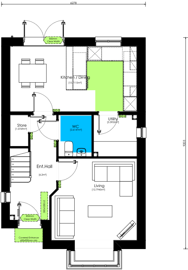
Ground Floor Plan scale 1:100
