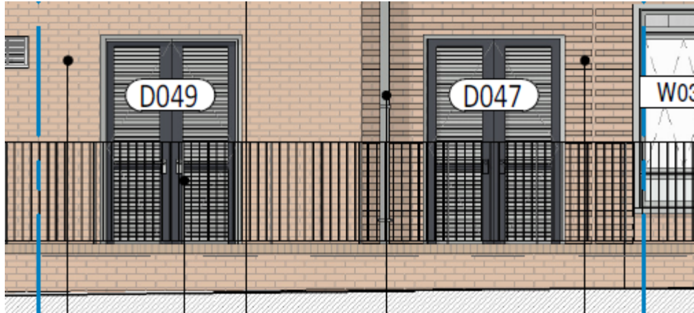
Figure 2 - Previously approved fully louvered openings (northern elevation)
