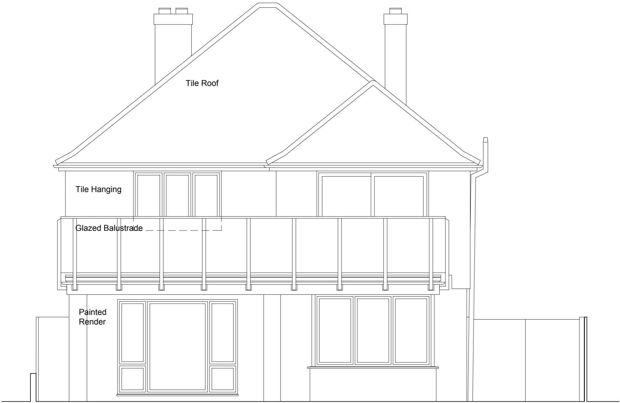
Existing Front Elevation (South) 1:50
