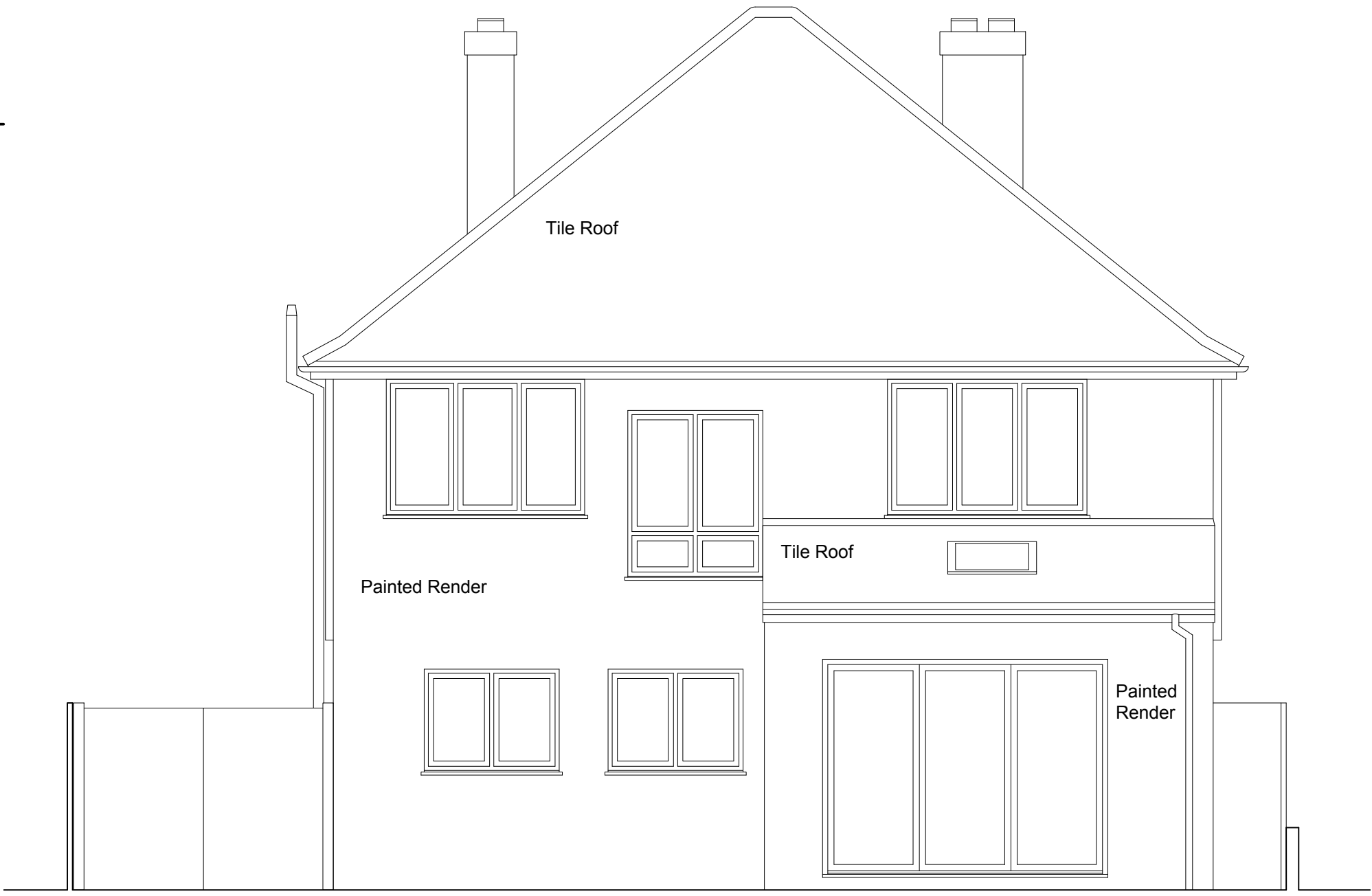
Existing Rear Elevation (North) 1:50
