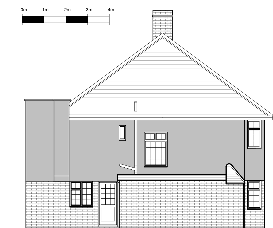
EXISTING NORTH ELEVATION 1:100
